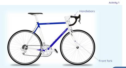
The handlebars are connected to the front fork. Moving the handlebar allows the rider to steer the bike. This could be called the steering **syste**l
